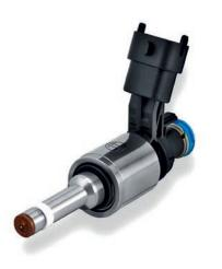
The HDEV 5.2 is a high pressure injector, which is developed to be used as a port or a direct injector. The function of the HDEV 5.2 is both to meter out the fuel and to obtain a well-defined mixture of fuel and air. It is an inward opening solenoid injector which is optimized regarding very short opening and closing times which ensures a very stable linearity at short injection times.
