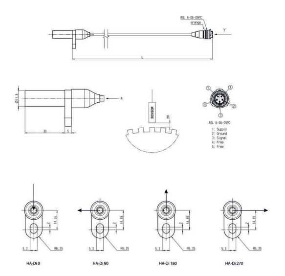
Direction of rotation of the target wheel, View A
